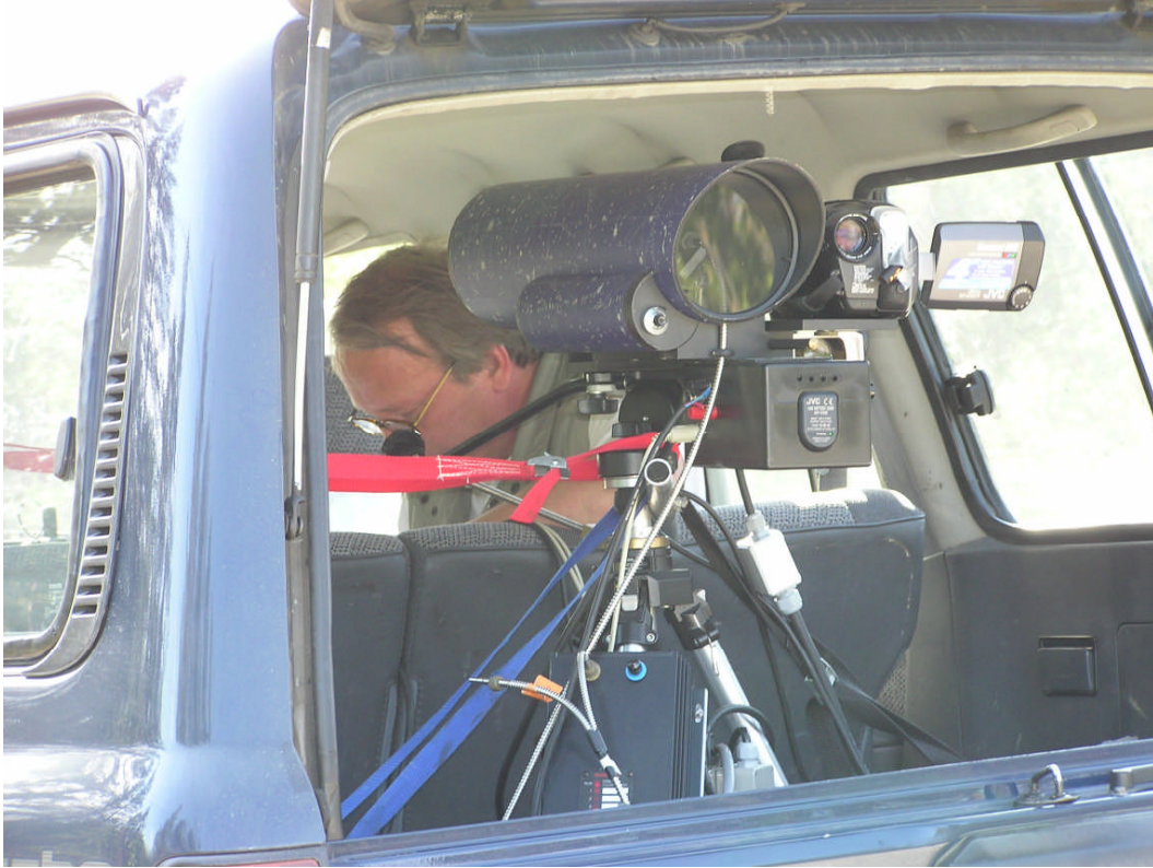
Figure 22. Field measurements using the optical spectrometer (Photo: Finnish Meteorological Institute).
